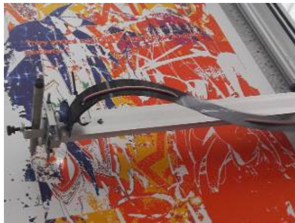
Figure 4 The pen-plotter's mechanical arm, equipped with a pen, is in action.
